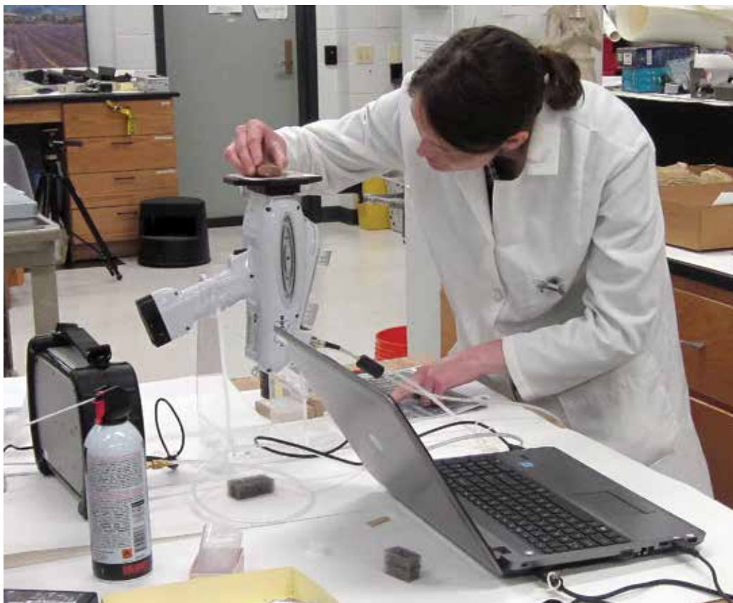
Figure 6. Probing the material support of the Archive: conservator Simona Cristanetti scans a Persepolis Fortification tablet with the portable X-ray fluorescence apparatus
