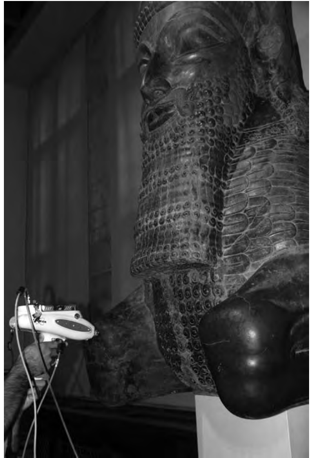
Figure 6. XRF analysis is carried out on a limestone column capital from Persepolis (OIM A24066; Achaemenid period; 486–465 B.C.)
