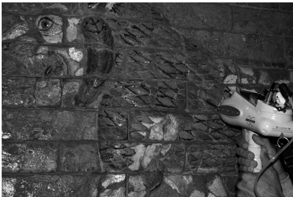
Figure 5. The hand-held XRF is used to analyze a glazed-brick lion from Babylon (OIM A7481: Neo-Babylonian period; 604–562 B.C.)
