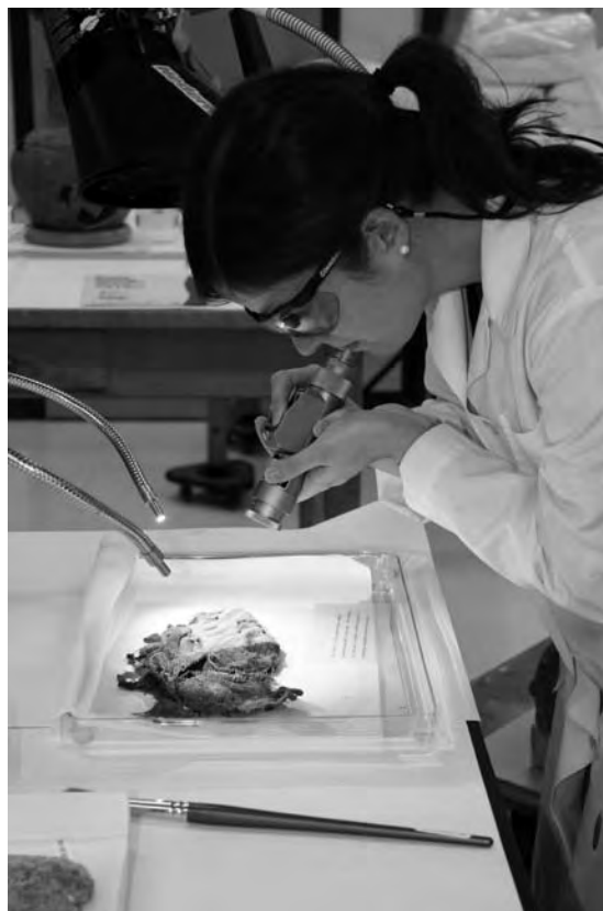
Figure 1. Alison Whyte, Assistant Conservator, tests the ability of the Class 4 laser to clean dark soil from the fragile surface of a textile excavated from Nubia
