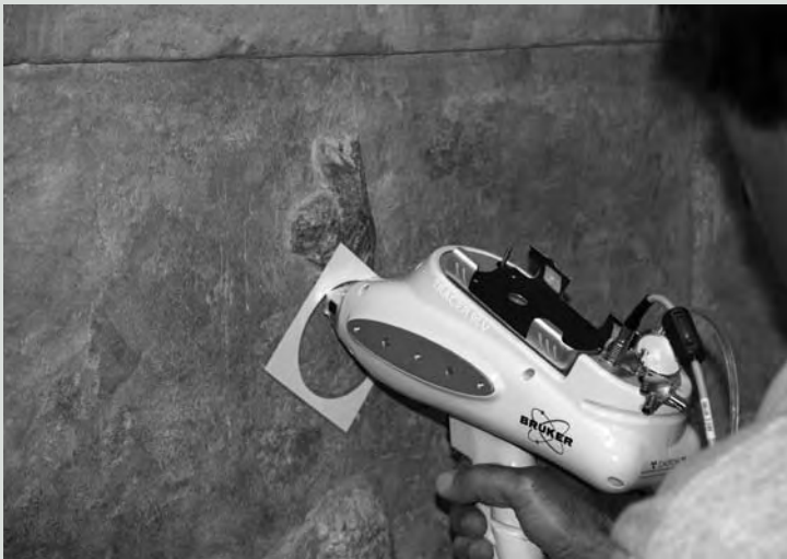
Figure 7a. The hand-held XRF is used to analyze the blue pigment present on the surface of one of the Room 7 Reliefs from the Palace of Sargon II, Khorsabad, Iraq (OIM A11255; Neo-Assyrian period; 721–705 B.C.)
