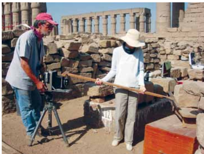
FIGURE 3.4. Photographer Yarko Kobylecky using a large-format camera in the blockyard of Luxor Temple. Photographic assistant Ellie Smith holds a measuring device that is exactly the distance necessary for a 1:5 scale photographic image and that also enables the camera lens to be completely parallel to the subject to eliminate distortion (photo by W. Raymond Johnson)
